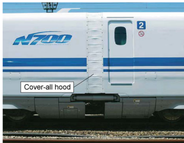
Fig. 8 Cover-all hood used in N700 series Shinkansen car (Central Japan Railway 2009b)
