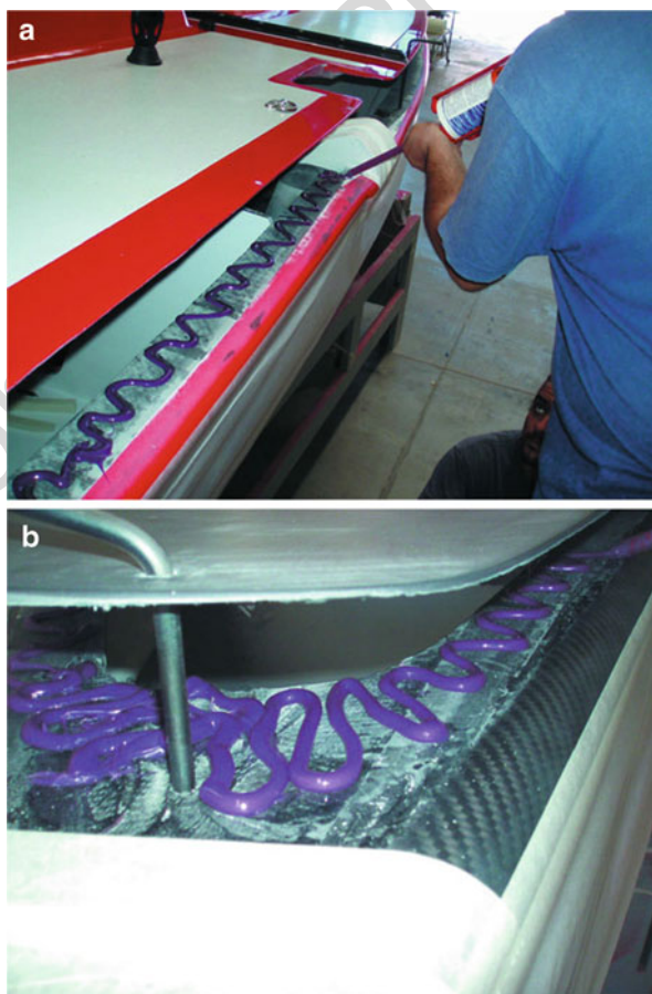
Fig. 4 Hull to deck assembly using a polyurethane adhesive. (a) Adhesive placement, (b) guide pin to ensure alignment (Photos Sika), (Sika 2009 )
