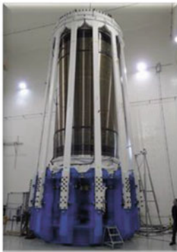
Static test on scale-one motor case to test the adhesive vessel/skirt joint (ASL)
