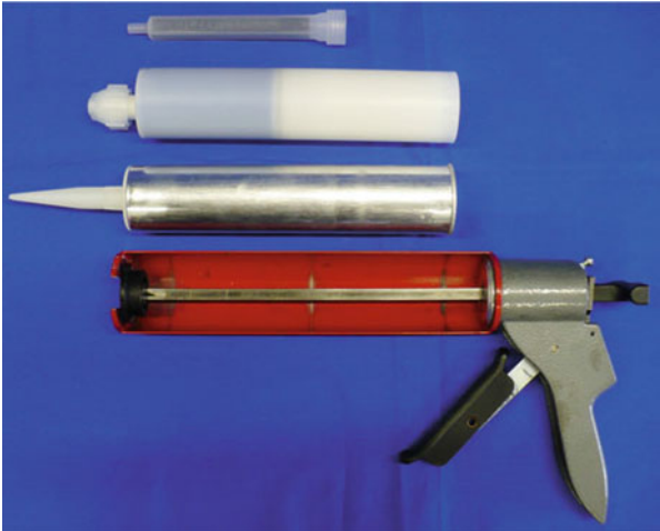
Fig. 11 Cartridge gun, plastic nozzle, aluminum cartridge for dispensing of one-component adhesives and mono-cartridge for dosing two-part adhesives
