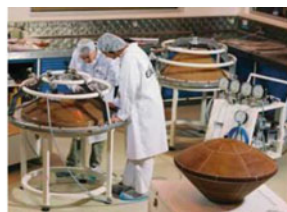
Beagle 2 heat shield assembly (ASL)
