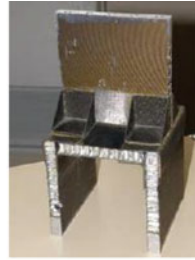
b) Wedges glued on sandwich panel (Courtesy Airbus Satellite)
