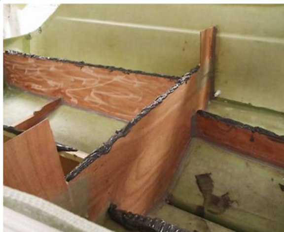
Fig. 3 Adhesively bonded marine plywood bulkhead in 6 m motor boat
