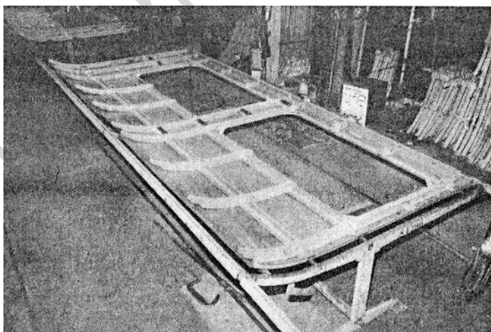
Fig. 20 The arrangement of the bodyside module components of suburban coach on the assembly jig (Seeds 1984)
