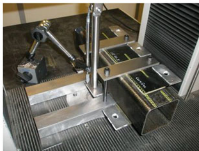
Bending test on elementary adhesive bond (ASL)
