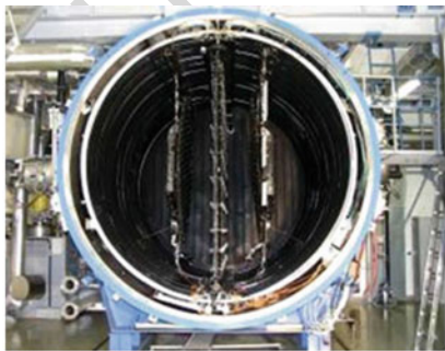
Thermal cycling with or without vacuum of the reflector (ASL)
