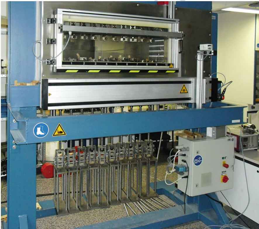
Fig. 9 Multi-sample tensile creep tester with video extensometer
