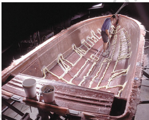
Fig. 2 Placing adhesive before bonding internal motor boat structure (Photo Plexus)
