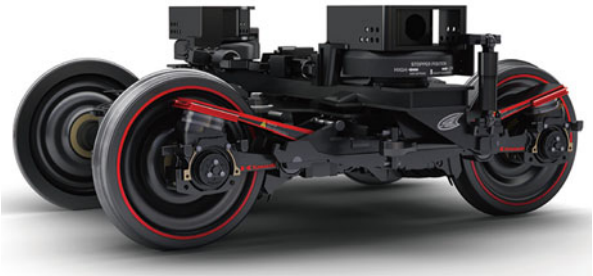
Fig. 10 Carbon fiber reinforced plastic (CFRP) bogie (Nishimura 2014)
