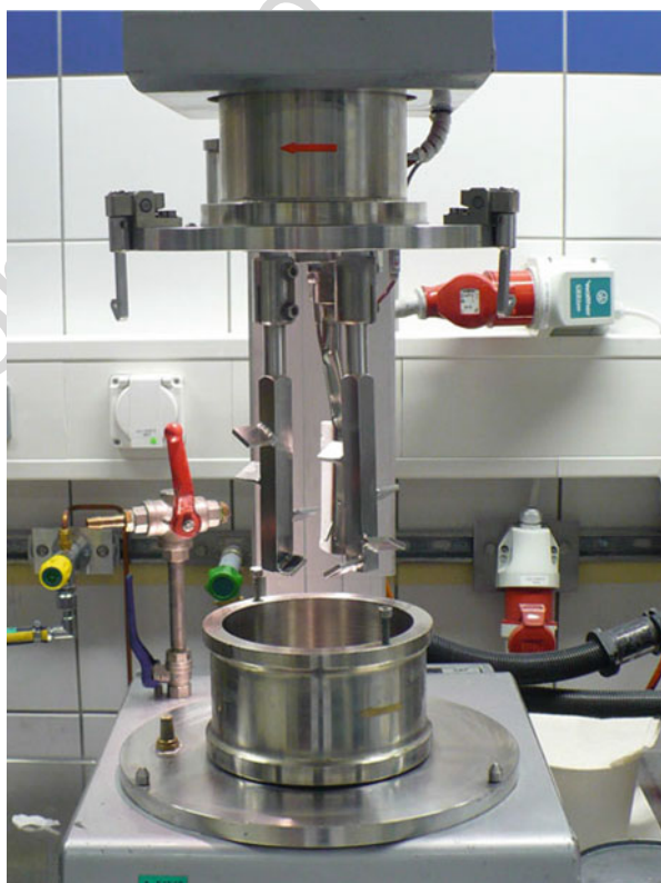
Fig. 2 Lab mixer with lift and planetary agitators, used to formulate adhesive samples of about 400 g
