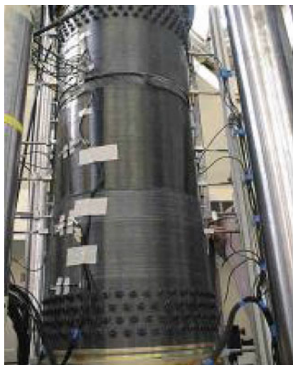
Reduced scale structure loaded in tension to validate the performance of adhesive skirt / vessel junction (ASL)
