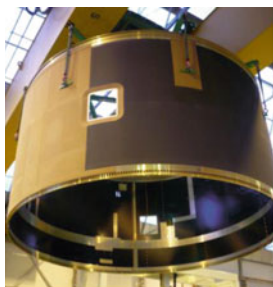
a) Thermal protection of interstage with cork panel
