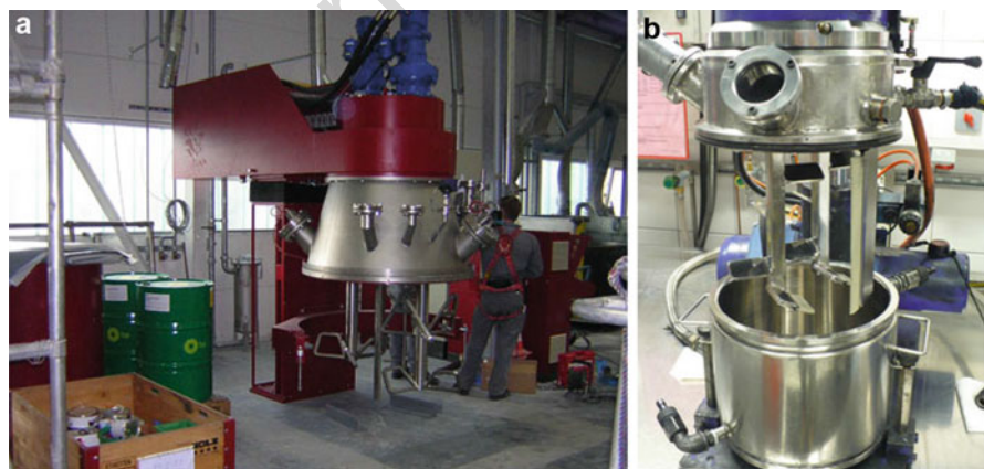
Fig. 3 Head and agitators of a planetary mixer which are used in production (a) and in a laboratory (b) to mix adhesive formulations. Butterfly agitators are used for the manufacturing mixer and finger blade agitators for the laboratory mixer. The production mixer has a volume capacity of about 1 t and the laboratory mixer of about 10 kg
