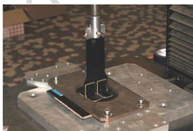
Out-of-plane strength to failure test on elementary bonded cleats (ASL)
