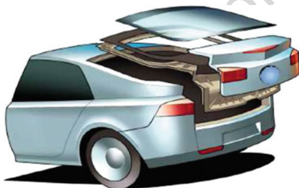
Fig. 6 Application of a dismantlable adhesive with thermally expandable microcapsules and blowing agents in the car industry, the ECODISM project (Papon et al. 2008)
