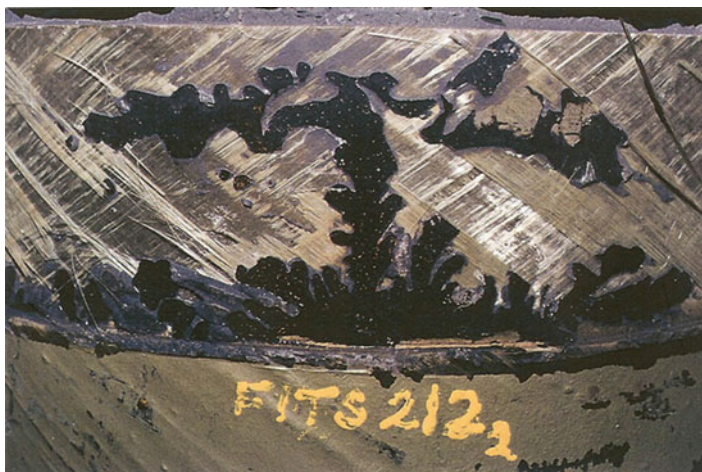
Fig. 6 Void in adhesive bond line most probably caused by moving the joint before the adhesive had reached a sufficient state of cure
