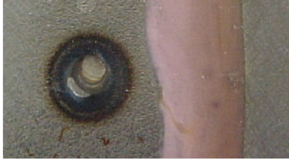
Fig. 23 Spot-weld sealed by using a two-part adhesive
