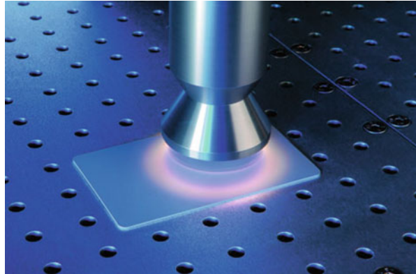
Fig. 31 Atmospheric plasma treatment of a polypropylene surface (Source Plasmatreat GmbH, Germany)
