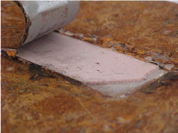
Fig. 22 Adhesive bond line after salt spray testing
