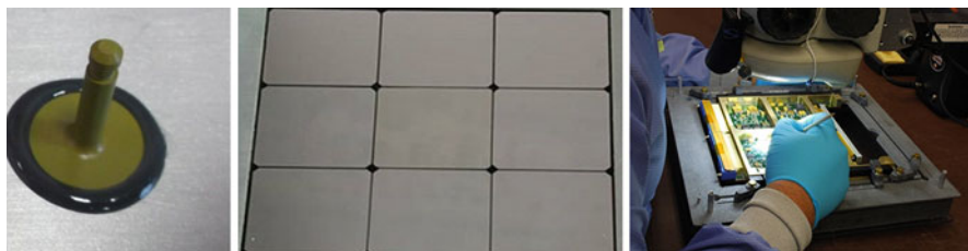
Fig. 3 Examples of adhesive use on spacecrafts: bonded stand-off for MLI (multilayers insulation) blankets mechanical installation on spacecraft structure ( left ), optical surface reflectors bonded on spacecraft structure for thermal control purpose ( middle ), electronic PCB proceeds through “touch up” after completing frame bonding, which uses a new automated adhesive dispensing process (NASA.gov image) ( right )
