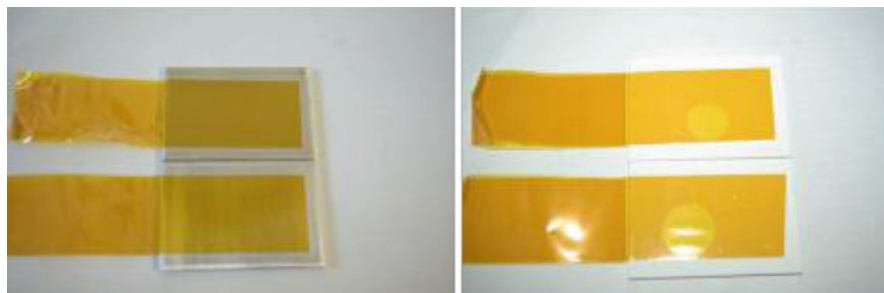
Fig. 19 Bubbles creation on an acrylic transfer tape due to irradiation (before irradiation on left / after irradiation on right ).
