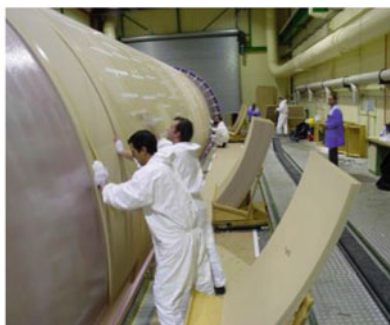
c) Ariane 5 cryogenic tank –thermal insulation bonding (CRYOSPACE image)
