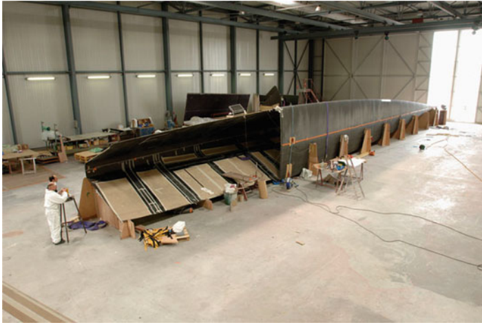
Fig. 9 Racing trimaran central hull halves during assembly
