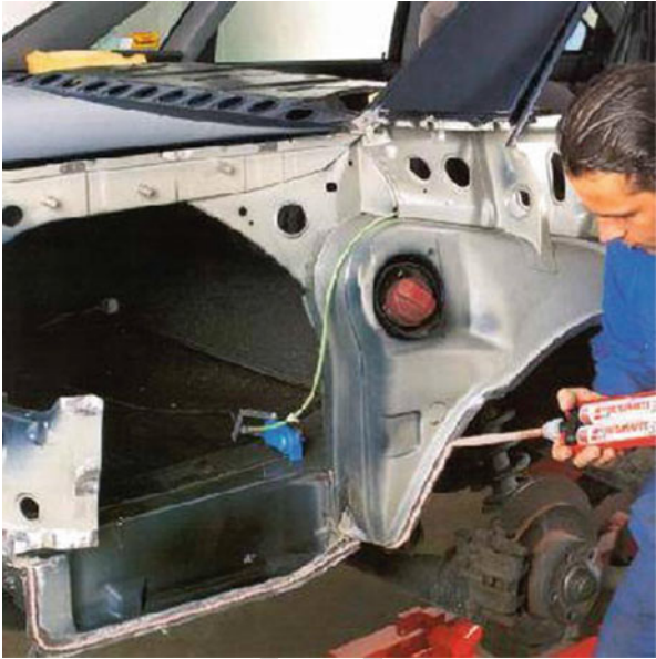
Fig. 21 Application of a two-part epoxy adhesive used for the body repair of cars
