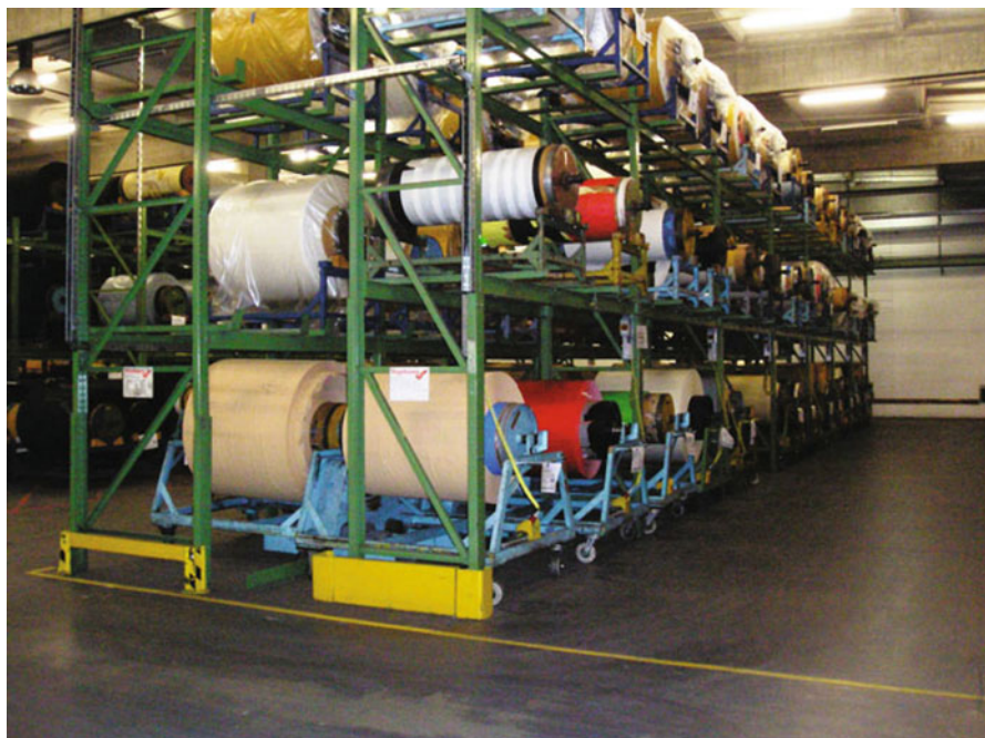
Fig. 2 Rotating racks for adhesive jumbo rolls in a temperature-regulated storage hall (Photo: tesa Werk Offenburg)
