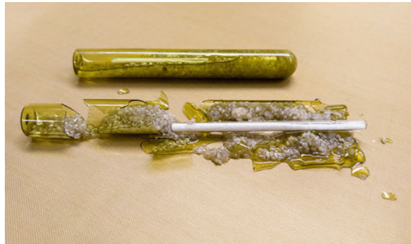
Fig. 2 Partly destroyed glass capsule for bonding anchors. The small glass tube contains the curing agent (Source: tff)
