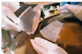
Bonding of cork tile on Beagle 2 front shield (ASL)
