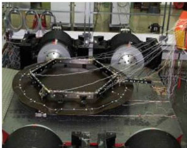
Dynamic tests of an antenna reflector (ASL)
