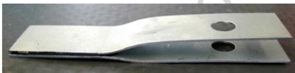
Fig. 19 Impact peel test specimen
