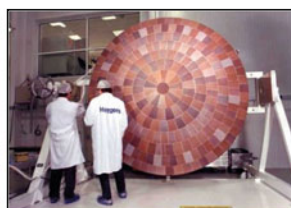
Huygens front shield 2.7 m in diameter, 60 half-angle conic spherical tiles (ASL)
