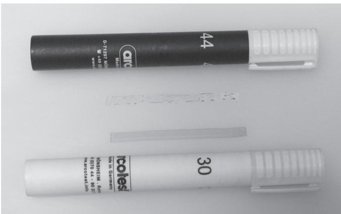
**Figure 6.1** Dyne pen test used for quality analysis of the surface energy.
