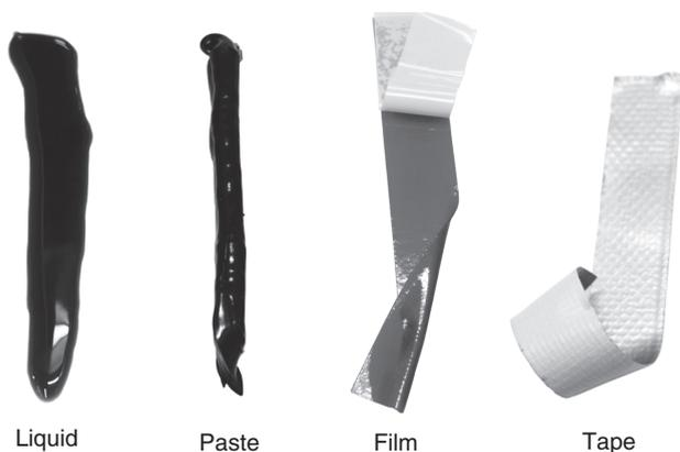
**Figure 4.6** Examples of the four main forms of adhesives.
