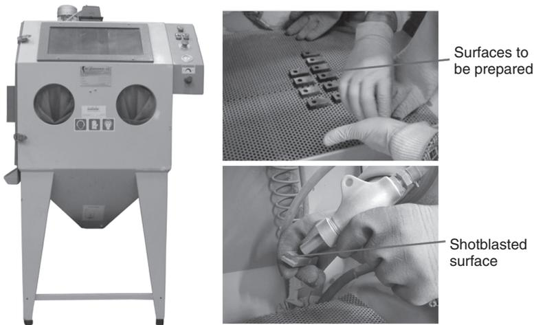
**Figure 3.7** Surface preparation using shot blasting.
