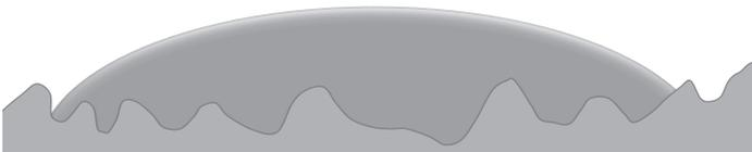
**Figure 2.5** Schematic representation of a liquid wetting a rough surface.
