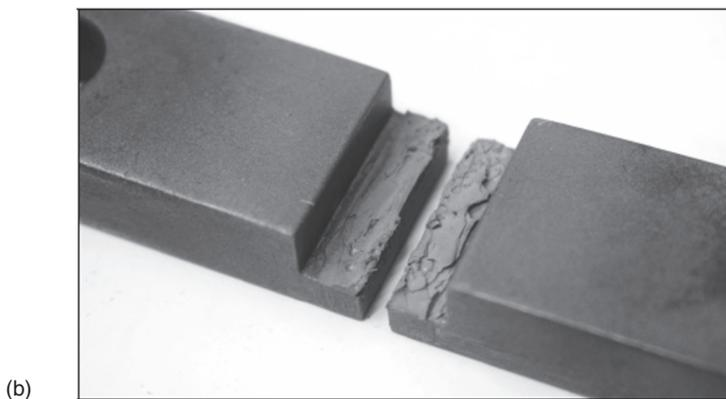
**Figure 4.12** The TAST specimen geometry ((a) dimensions in mm) and an example of a successfully tested specimen (b).
